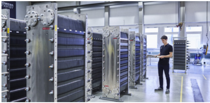
Growing market: highly efficient electrolyzer stacks
